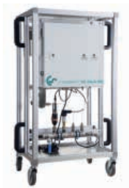
Compressed air quality measurement
