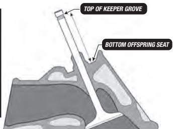
Diagram 1. Calculating Installed Spring Height
