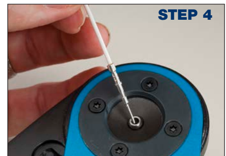
REMOVE TERMINATED WIRE ASSEMBLY
