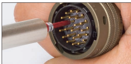
Typical application showing tool testing pin contacts.
