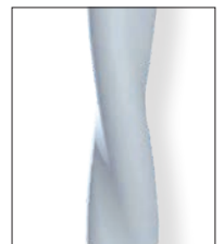
LEFT HAND LAY "S" DIRECTION
