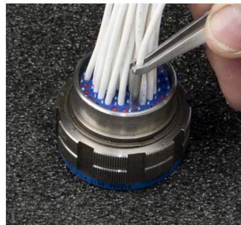
Typical All Metal Tool Operation
