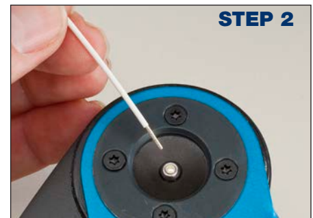
INSERT PRE-STRIPPED WIRE
