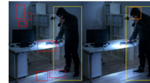
DL Object Tracker Only triggered based on an objects classification (e.g. person, vehicle)
