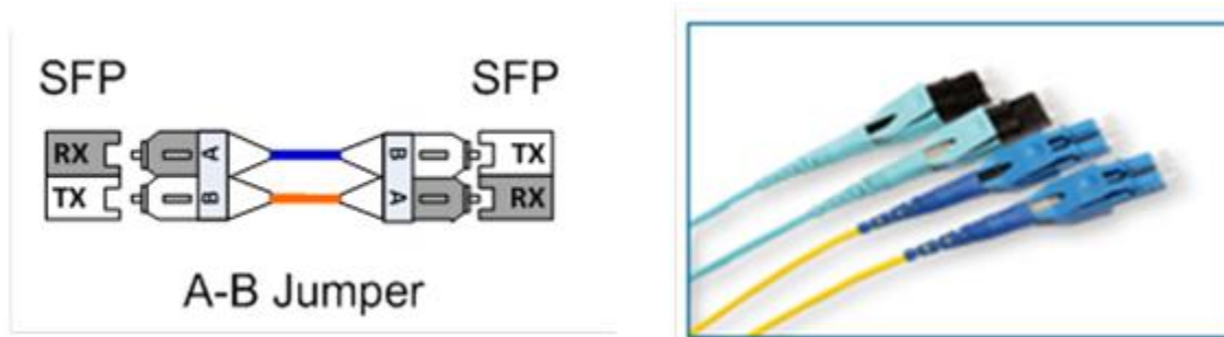
Figure 1: Duplex Fiber Optic Transmission
