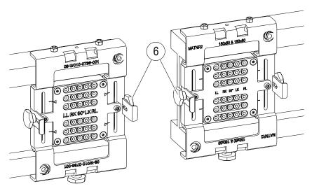
Fig. 9: Left stop and right stop
