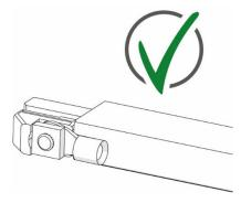
Fig. 43: Correct position of the clamping unit
