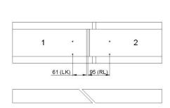
Fig. 31: 45° rail stop tapering to the left
