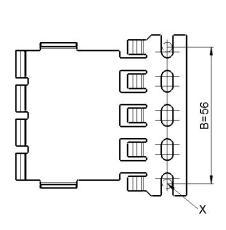
Fig. 5: Installation plate, 4 pole
