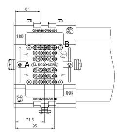
Fig. 13: Distance between the rows and the stop plates (right)
