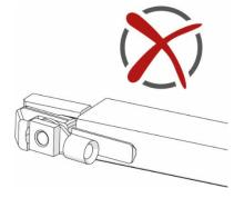
Fig. 44: Incorrect position of the clamping unit
