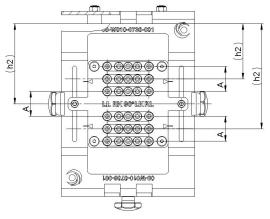
Fig. 34: Drilling jig spacing "A"
