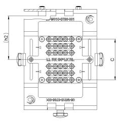
Fig. 36: Drilling jig spacing "C"
