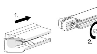
Tighten the end cap with a 3-mm hex screw-driver to **2 Nm**.
