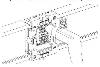
Fig. 39: Drill the first hole
