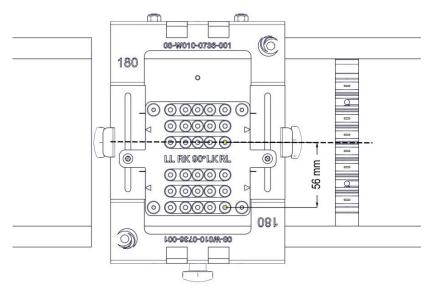
Fig. 40: Align the drill bushing block
