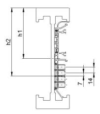
Fig. 10: Installation plate on a guideway profile
