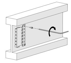
Fig. 3: Drilling an EMS guideway profile using a drilling jig
