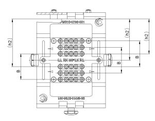
Fig. 35: Drilling jig spacing "B"
