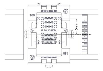
Fig. 38: Align the drill bushing block
