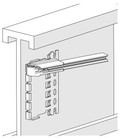
Fig. 45: Hooking the conductor rail in place
