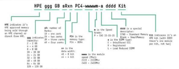
HPE 8 GB 1 R-4 PC4-2133P-R STND Kit indicates an HPE Standard Memory DIMM with a 8 GB capacity, single rank, a data width of 4, memory type of DDR4, 2133 registered, 15-15-15 latency, and an HPE kit.
