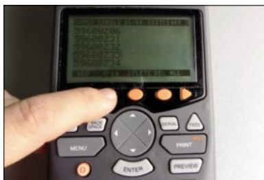
Step 1) Turn on unit, press the FILE button and select one of the many pre-saved templates.
