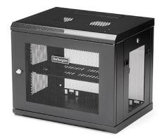
This 9U server rack cabinet lets you mount your EIA-310 compliant equipment to the wall. The enclosure features an adjustable mounting depth from 6 to 15 in. and offers a maximum load capacity of 200 lb. (90 kg).
