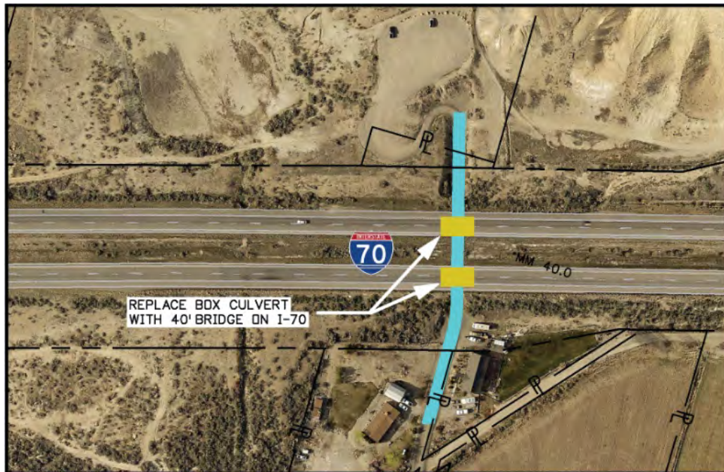
Alternative 8: Replace Culvert – Two-Lane Bridge
