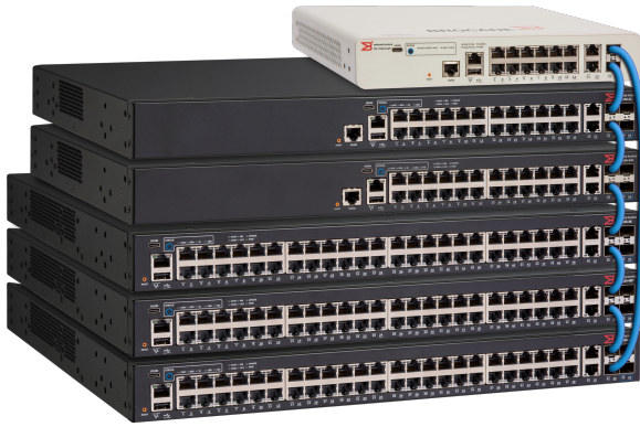
Figure 3. Up to eight Ruckus ICX 7150 switches can be stacked together into a single logical switch using standard SFP+ 10 Gbps ports and copper cables or optics.
