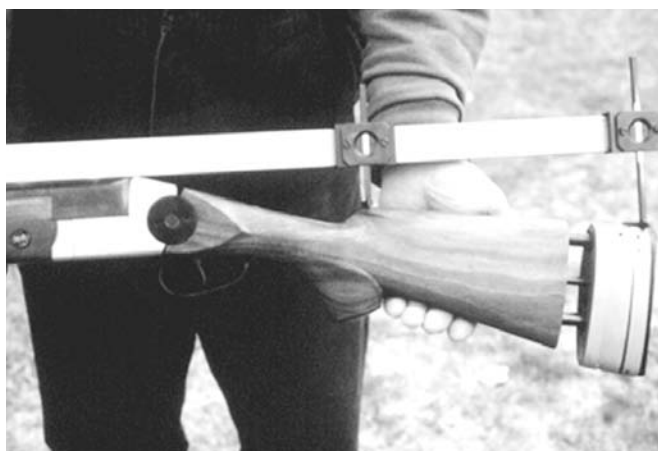
Graduated gauges allow accurate measurement from the reference bar
