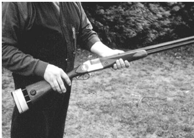
The Merkel Try Gun has no internal functioning parts, but multiple external adjustments
