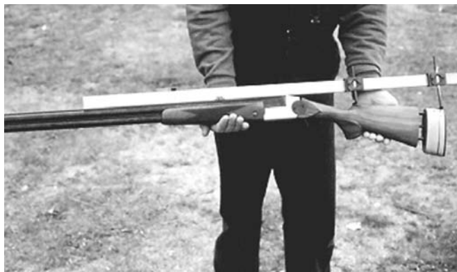
The aluminium straight edge fixes to the rib to provide an indexing reference for all the stock measurements
