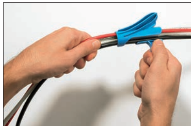
Insert one or more cables into the insertion slot of the applicator tool.
