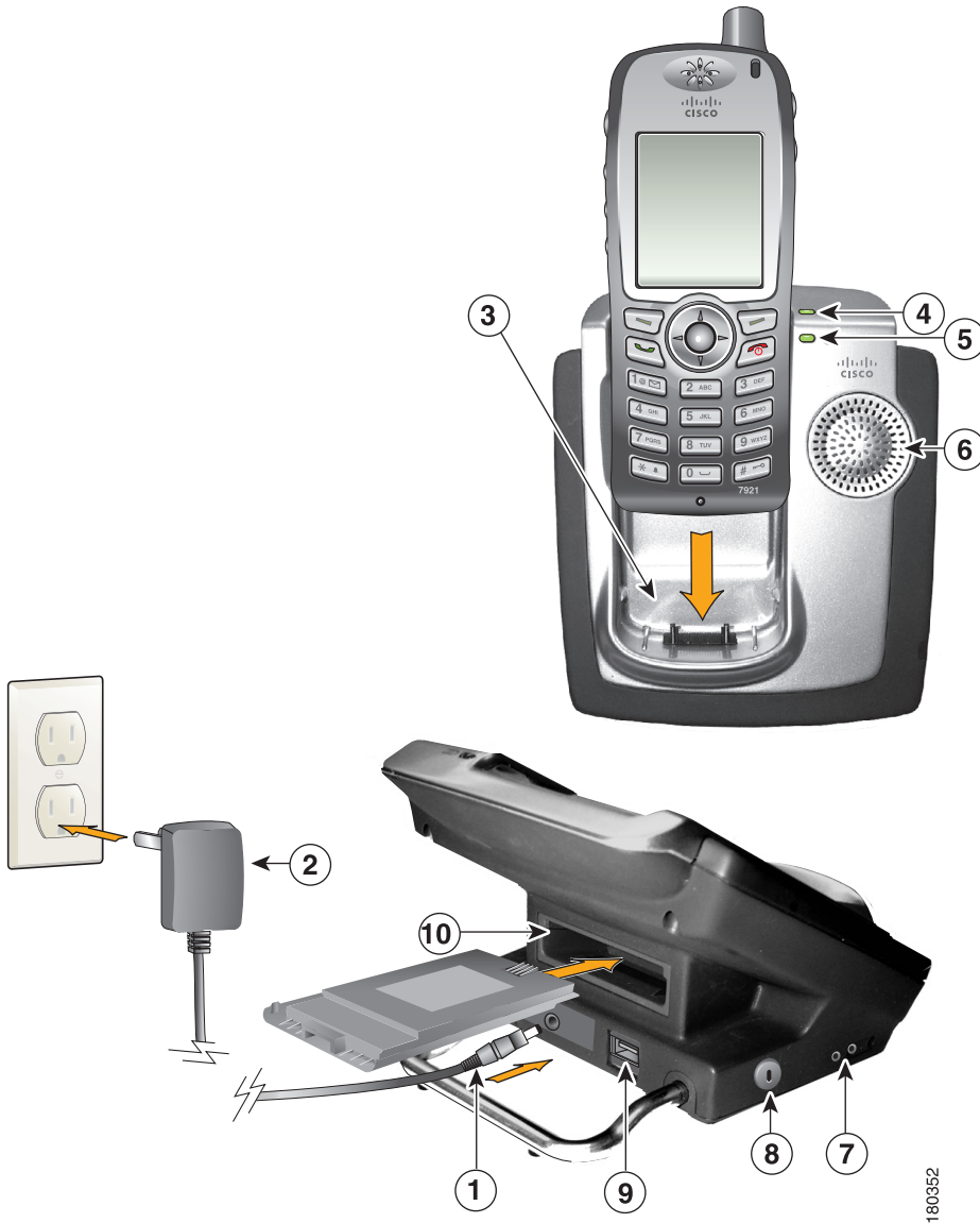
Figure 3-5 Desktop Charger Assembly and Components
