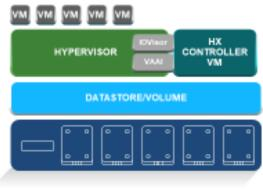
HX Controller VM Assumes Direct Access of Local Storage IOVisor Module Presents Pooled Storage to HyperVisor and Stripes IO Data Services are Offloaded to HX Data Platform
