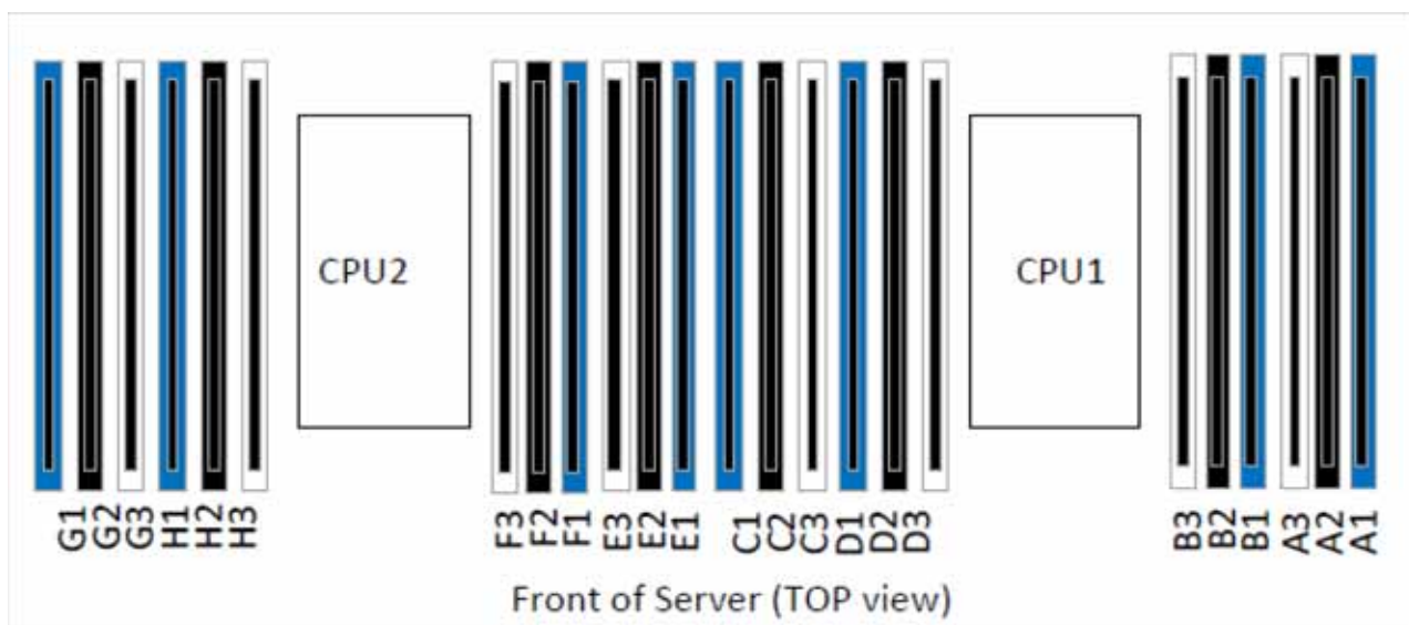
Figure 8 Physical Layout of CPU DIMM Channels and Slots
