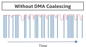
As shown by the red line, components have less time between DMA calls to reach and stay in lower power.
