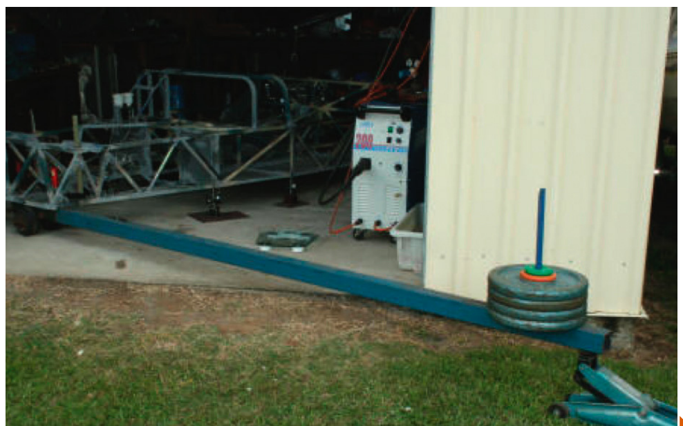
You can measure your chassis stiffness with a simple tool such as this, which constrains the chassis at a suitable point
