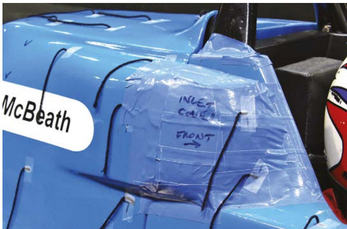
A fairing placed over the engine inlet made a useful difference, but would be impractical
