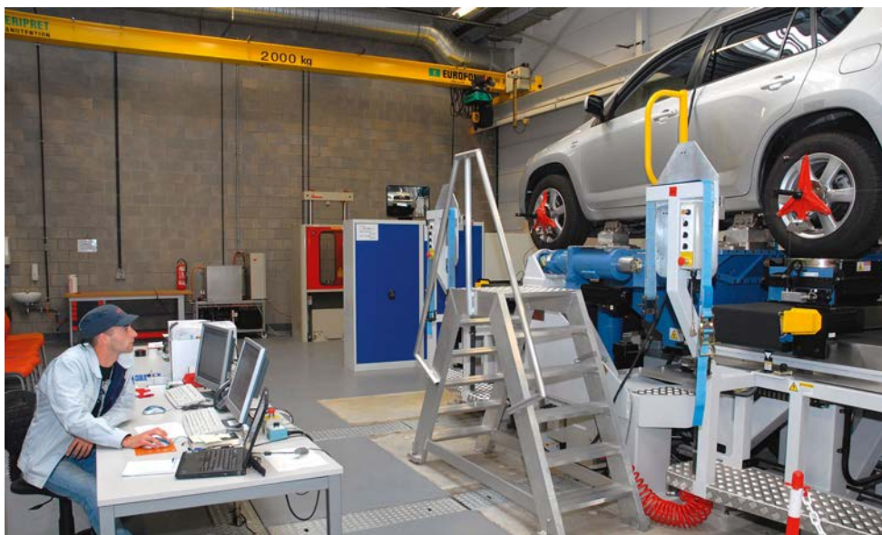
K&C rig time is expensive and they are often used by manufacturers (this belongs to Toyota) but there are other solutions
