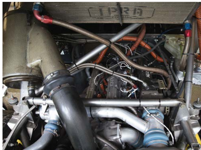
The engine made use of a supercharger and a turbocharger, the former for negating the turbo lag out of corners, the latter for high end revs at full chuff
