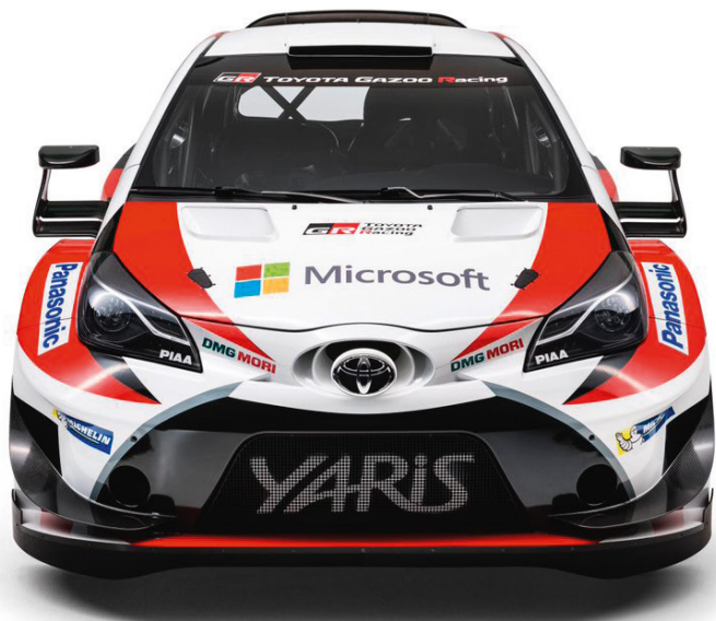
The splitter has received much attention. Thanks to the allowance of multi-layer carbon for aerodynamic devices this is now strong enough to survive the rough special stages
