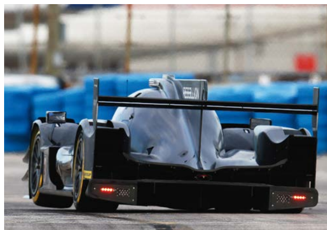
Sebring's challenging Turn 1 is bumpy, slippery and fast, and is a true test for both the tyre and the racecar set-up. Every one of the new LMP2s adopted this inside-front lifting attitude around this particular corner on the first day of the test
