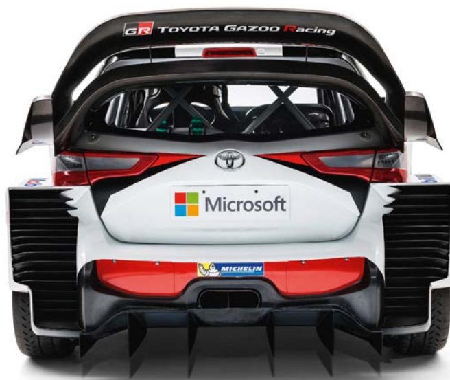
New regulations allow plenty of freedom in diffuser design while it can now protrude beyond the bumper by 50mm. Rear wing is dramatic, just as the new rules intended
