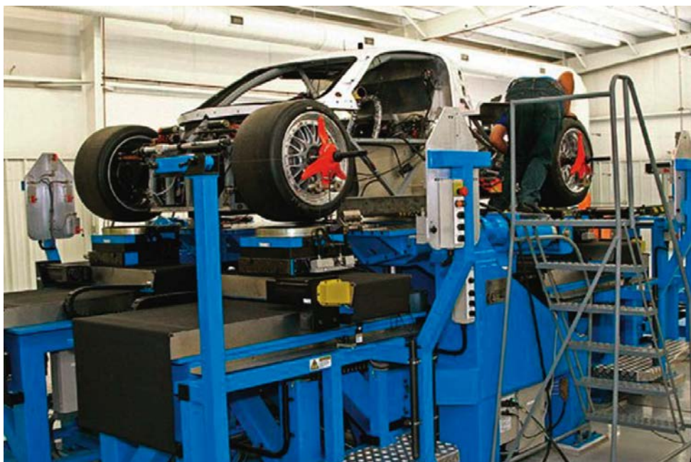
Kinematics and compliance rigs (K&C) are an ideal way to check over a car's chassis without running it on the race track
