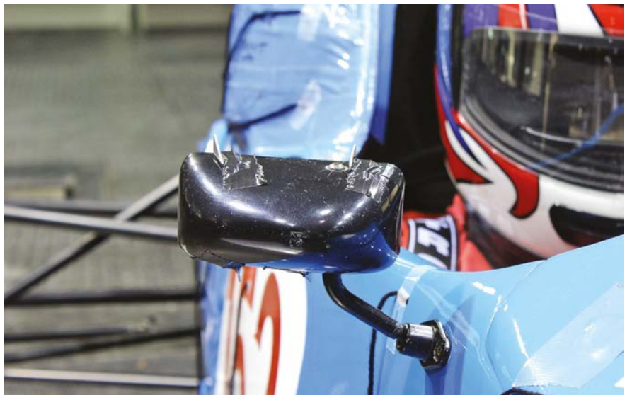
Small vortex generators were fitted on the car's mirrors with the object of reducing the size of their wake
