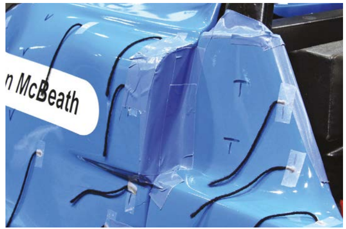
Taping directly over the Swift's inlet duct actually made no difference to the drag
