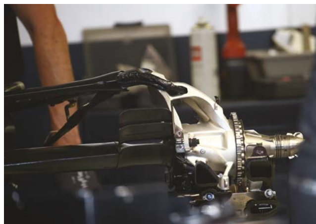
Rear upright with brake cooling parts. Suspension at the back is pull rod design
