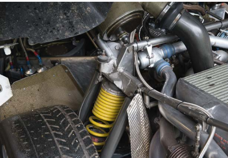
Suspension was double wishbones and coil springs with single telescopic hydraulic shock absorbers at the front while twins were fitted at rear. Little was carried over from the 037
