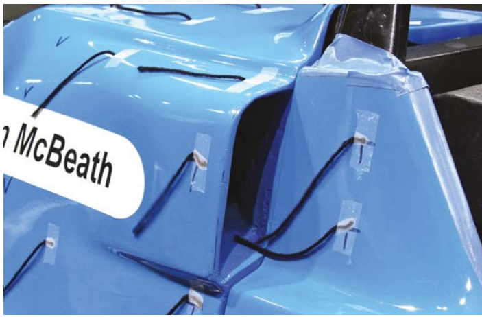
The object of one of our experiments was to find out if the engine inlet duct created drag
