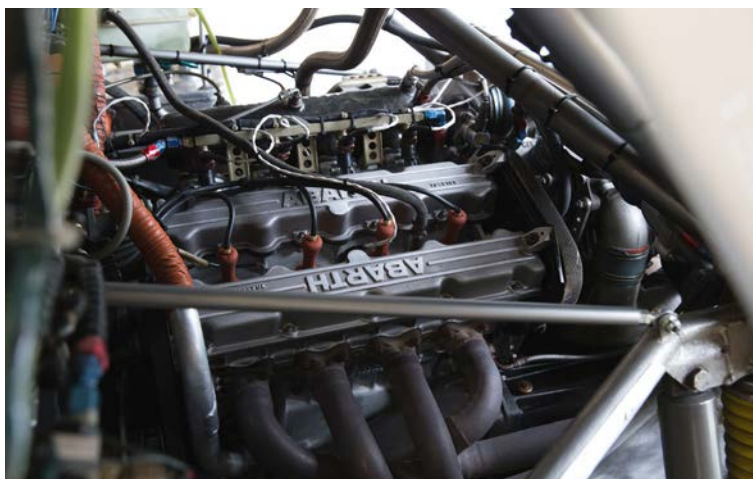
The 1759cc 4-cylinder powerplant was brand new and both the block and the head were constructed from lightweight aluminium alloys. The head featured twin overhead camshafts
