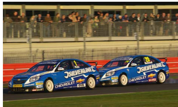
Brief rear wheel lock-ups, as on the second of these two touring cars, are a natural characteristic of front-wheel-drive racecars
