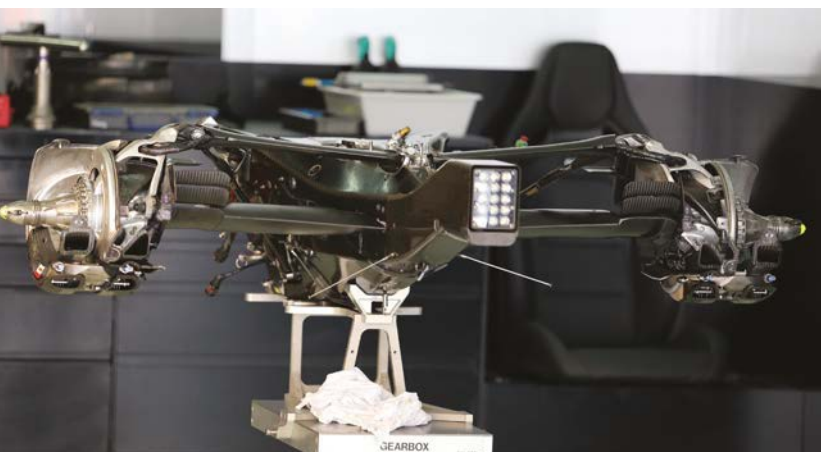
Semi-automatic gearbox features a composite outer skin around a titanium inner cassette
