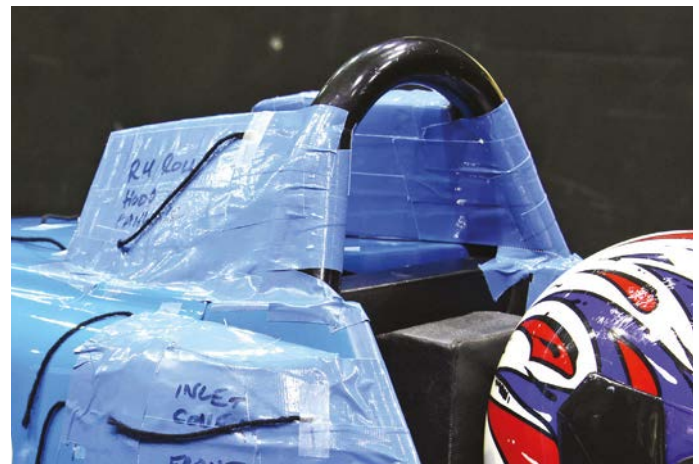
These roll hoop fairings were one of the most beneficial modifications of the session
