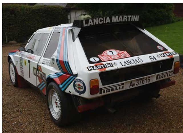
A carbon-fibre composite body ensured the S4 tipped the scales as close to the minimum weight as possible. C-pillar scoops fed air to intake and intercoolers
