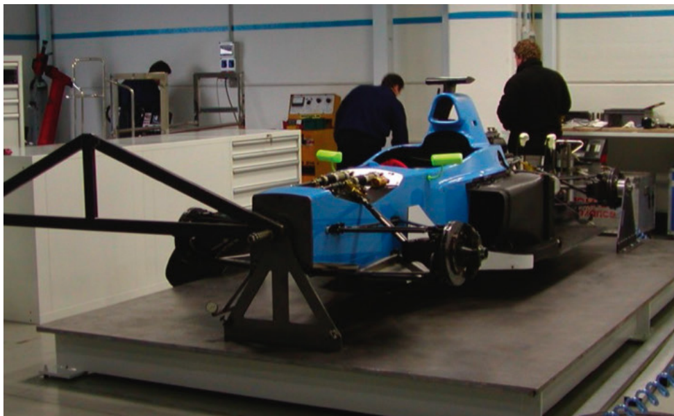
This is a more sophisticated approach to checking the torsional stiffness of a racecar, this time applied to a Lola B02/50
