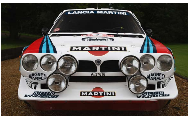
While the aero was rudimentary, with up to 550bhp on tap at high boost settings the large chin spoiler was vital for keeping the nose down at high speed. The light cluster possibly helped too!
