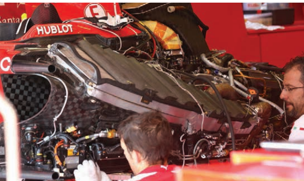
Plenum is smallest in F1, suggesting 059/4 does not feature variable inlet. Wastegate configuration has changed from 2014
