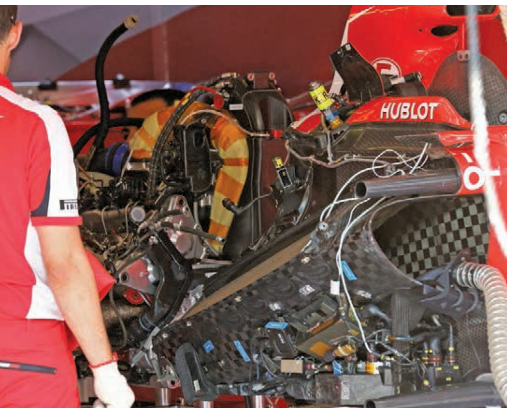
059/4 power unit installation – this picture graphically illustrates the mind-boggling complexity of a modern Formula 1 car
