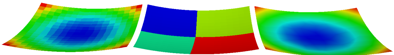
Figure 8. Exchange surface with additional information (left to right) - field received by Fortran (CHR_000*.case) - Fortran partitioning (from CWIPI output files) - filed sent by the C code (CWIPI output files)
