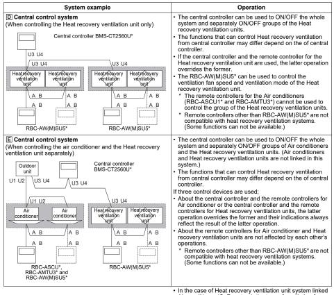
In the case of Heat recovery ventilation unit system linked Air conditioner (C, F system), the type of ventilation fan speed that you can select from the remote controllers are less than Heat recovery ventilation unit ONLY sysytem (A, B, D system). In the case of Heat recovery ventilation unit system linked Air conditioner (C, F system), the type of ventilation fan speed that you can select from the remote controllers are less than Heat recovery ventilation unit ONLY sysytem (A, B, D system).
