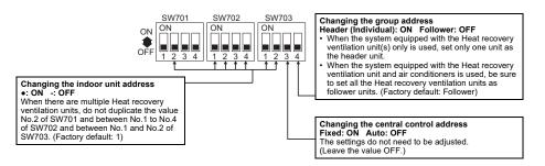
Indoor unit address switch (●: ON —: OFF)
