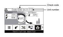
When a trouble occurs in the Heat recovery ventilation unit, the check code and the Heat recovery ventilation unit number flash on the display of the remote controller.
