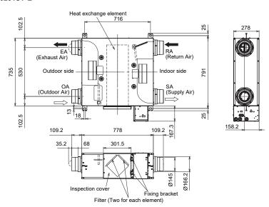
Weight: 29 kg Heat exchange element: 1
