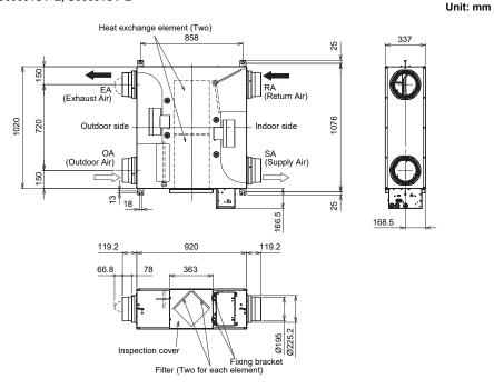
Weight: 47 kg Heat exchange element: 2
