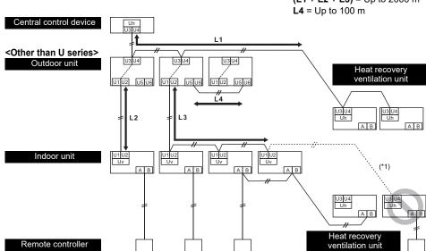
\*1. This connection is prohibited. Connect the Heat recovery ventilation unit (U series) with U3 and U4 line.
