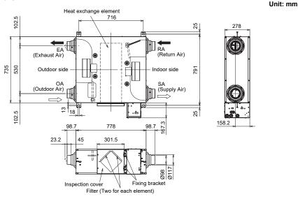
Weight: 29 kg Heat exchange element: 1
