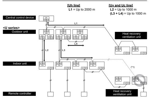
\*1. <u>This connection is prohibited.</u> Because central controller cannot recognize Heat recovery ventilation unit and cannot operate Heat recovery ventilation unit at all. (Heat recovery ventilation does not appear in central controller.)
