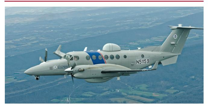
The Multi-Role Enforcement Super King Air 350ER (MEA) is a medium- range, fixed-wing, twin turboprop aircraft. It's used by U.S. Customs and Border Protection, Air and Marine Operations (AMO) to conduct aerial patrol and surveillance over land and water, and for enforcement relocation of personnel and equipment.
