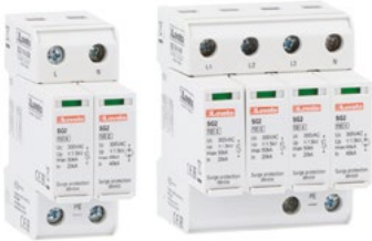
Overspanningsbeveiliging | SERIE SG Type 2 1P, 1P+N, 2P, 3P, 3P+N, 4P versies Beschermingsniveau Up (1,5kV) I max (8/20μs) 50kA of 15kA
