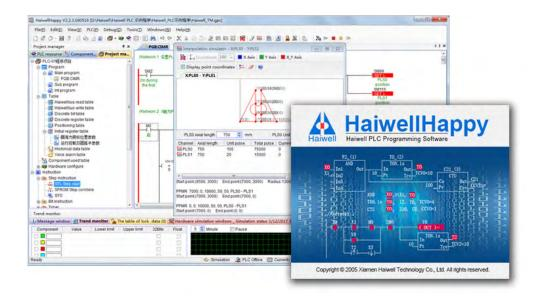
HaiwellHappy is the programming software for Haiwell PLC. It accordance with IEC 61131-3 standard, supports 100% built-in simulator and three kinds of programming languages (LD-Ladder Diagram, FBD-Function Block Diagram and IL-Instruction List). It can run on the systems of Windows 98, Windows 200X, Windows XP and the later Windows versions.
