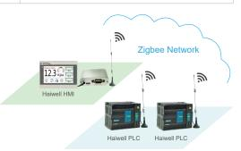
PC2ZB is a type of wireless communication expansion module that used on PC terminal. It convers PC terminal of RS232/RS485/ USB to ZigBee singnal. Through this module, HaiwellHappy can be online and read-write in wireless mode with the host PLC which is extended with H01ZB.
