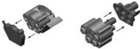
Figure 10 – Removal of Dust Caps img-00593 & img-00597
