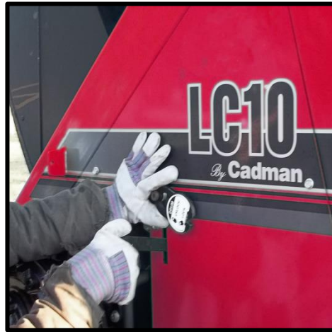
Figure 40 – Connect Break-Away Cable and Lock Prior to Transport
