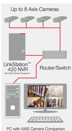
PC with AXIS Camera Companion for live viewing and configuration.
