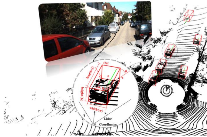
Figure 43 Visualization of object detection using 3D LiDAR data from (196)
