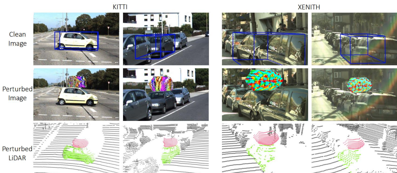
Figure 16 Exemplary visualization of an evasion attack on LiDAR and camera-based object detection from (47)
