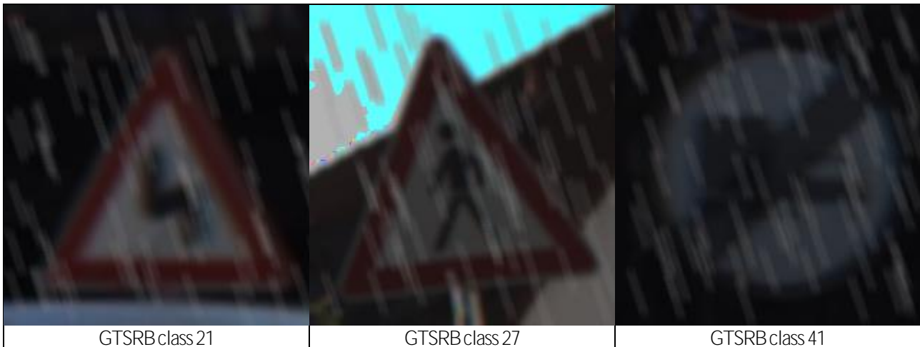
Figure 72 Exemplary images for class 21, 27 and 41 transformed by the heavy rain transformation
