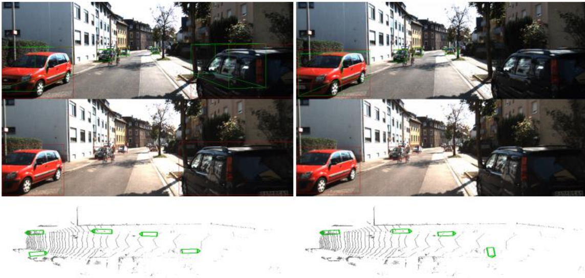
Figure 5 FGSM attack results on a 3D object detection system from (23). The images on the left contain the clean stereo image with the result of the 3D object detection underneath. The images on the right show the FGSM perturbed stereo image and the corresponding 3D object detection result underneath.
