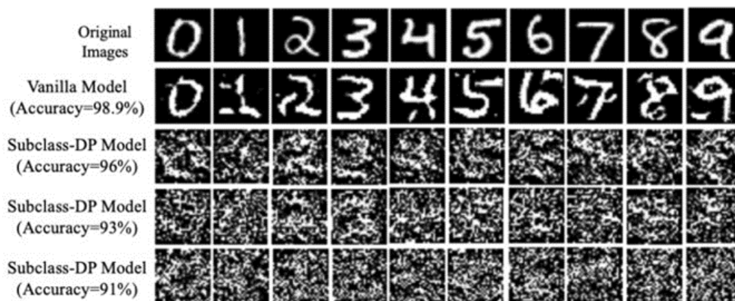
Figure 22 MNIST data set with different thresholds of added noise from (75)
