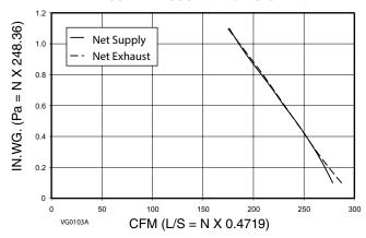
FULLY ADJUSTABLE SPEED RANGE FROM 50 CFM TO MAXIMUM SPEED.
