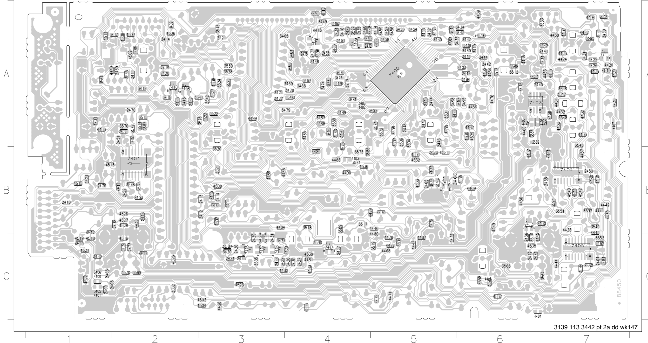
This assembly drawing shows a summary of all possible versions. For components used in a specific version see schematic diagram and respective parts list.
