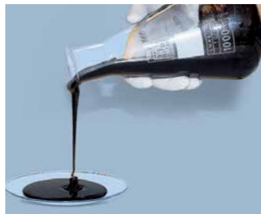
Aged engine oil With soot contamination, poor lubrication properties
