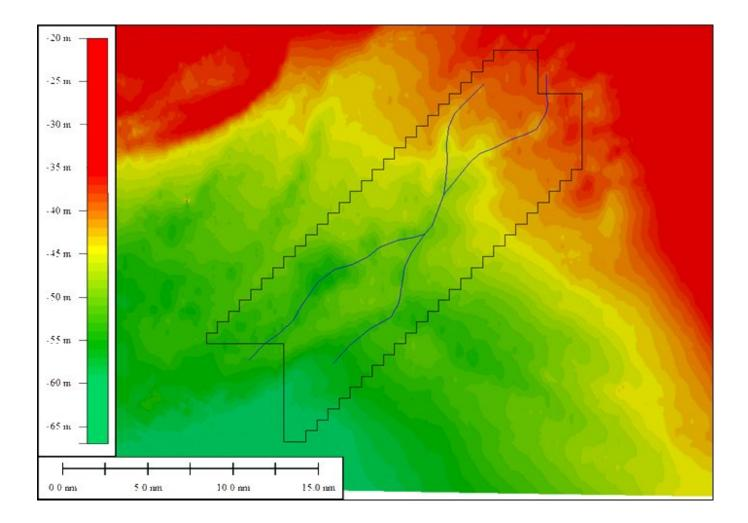
Vineyard Wind Lease OCS-A 0501 with surface features (blue trend lines) that could be inferred from the seafloor topography. Bathymetry from NOAA's coastal relief model dataset, approximately 90 m gridded depth points. <u>https://www.ngdc.noaa.gov/mgg/coastal/crm.html</u>. These features are extremely broad with low relief and no associated subsurface structures, not indicative of a preserved paleofeature.
