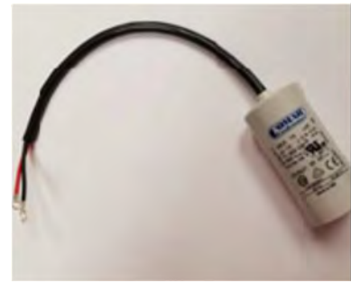
CB9 – Motor Capacitor for Mixing Room Fan
