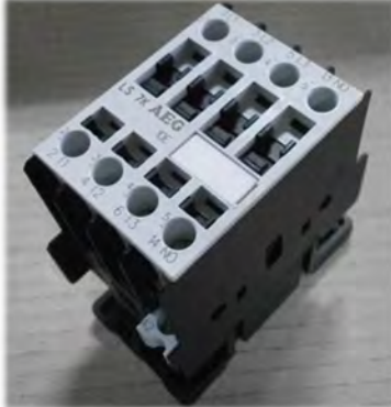
9TE0540 MOTOR CONTACTOR - 3P+1NO - 18A 230V - LS7K10-50
