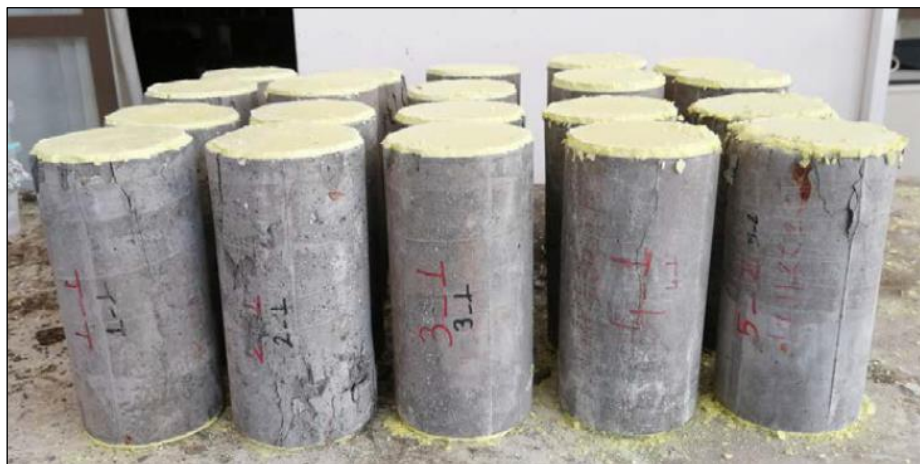
Figure 5. Pictures of SCC specimens after elastic modulus test.
