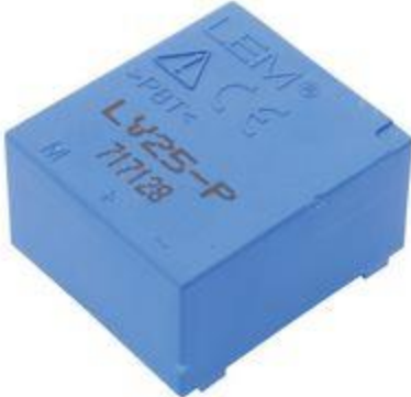
Figure 4. LEM-LV25P voltage transducer and its connection
