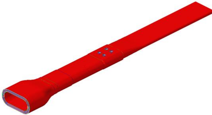
Figure 35. Output shape of torque tube after sizing optimization.
