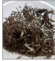
b) Basalt Fiber (Hanafi et al., 2020)
