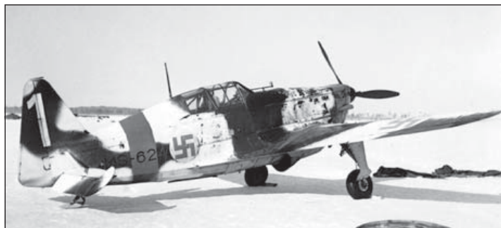
MS-624 of 2/LeLv 28, photographed at Hirvas whilst assigned to Sgt Uolevi Jaakkola, was temporarily painted in white winter camouflage on 20 February 1943. The whitewash 'recipe' employed by 2/LeLv 28 groundcrew consisted of casein glue mixed with chalk powder ( Erkki Jaakkola )
