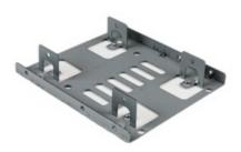
The BRACKET25X2 Dual hard drive mounting bracket kit enables you to maximize the internal mounting space of your computer, by installing two 2.5in SATA hard drives (HDD) or solid state drives (SSD) into a single 3.5in mounting bay. The bracket can be used with IDE drives using our 2.5in to 3.5in IDE Hard Drive cable adapter (IDE4044).
