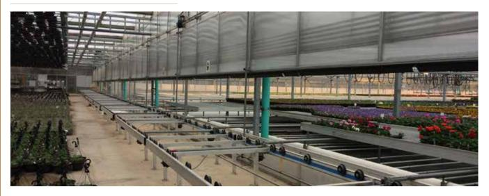
Ventilation is an essential component for the greenhouse growing environment. Types of ventilation can be forced air or passive ventilation. When designing a new greenhouse, we always take into consideration the passive ventilation incorporating roof & side vents to increase air flow and produce excellent quality crops.
