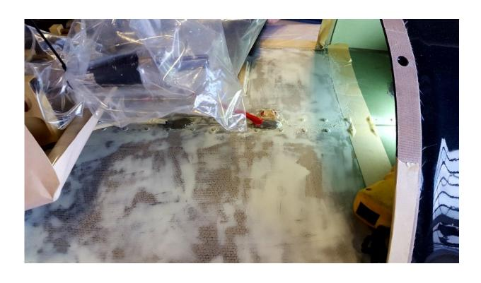
**Figure 6** – Finishing glaze compound (C-266) after sanding high spots results and when pin hole filler was used during manufacturing example.
