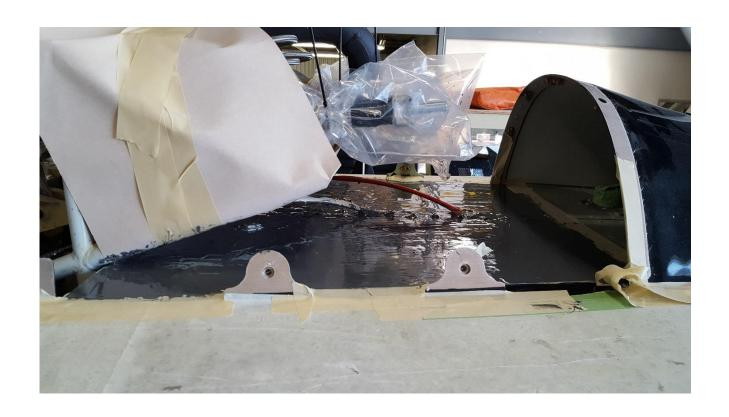
Sealant (C-322) applied on repaired surfaces.
