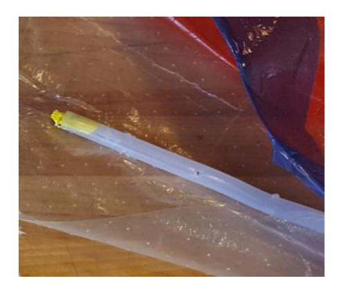
**View C**Holes drilled into the plastic tube material.
