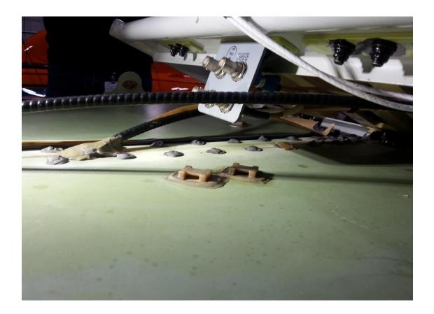
Figure 3 - Typical wicking stains (wet spots)
