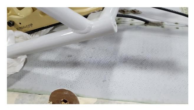
Signs of wicking appearing after wiping with the solvent mixture.
