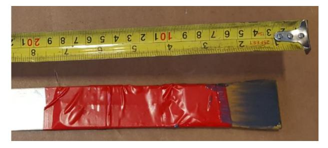
Plastic spatula (soft) cut to size used to spread sealant under the servo actuators.
