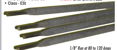
1/8" Run at 80 to 120 Amps DC Reverse Polarity (Electrode +) or AC
