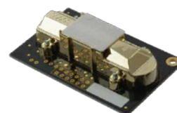
Sensor A (Can be field calibrated)
