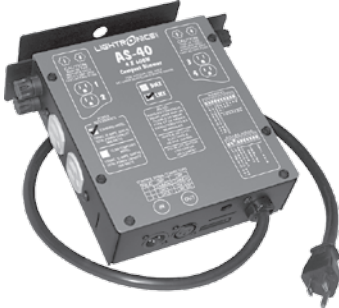
AS40L / D 4 Channels @ 600 Watts
