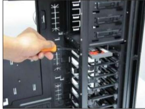
Secure your drive with the provided 2.5" screws.
