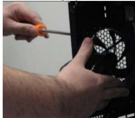
Unscrew the rear fan to remove it.
