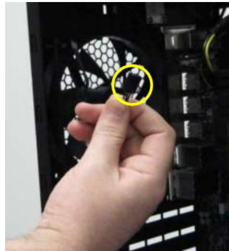
Disconnect the 3-pin power connector.
