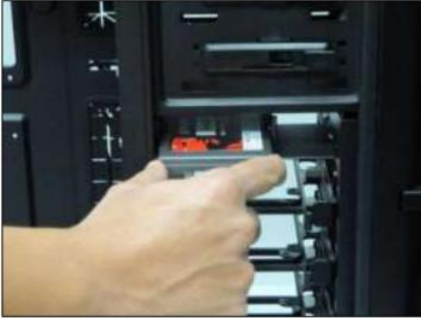
Slide your 2.5" drive into the drive bay so that the drive's holes align with the drive bay holes.
