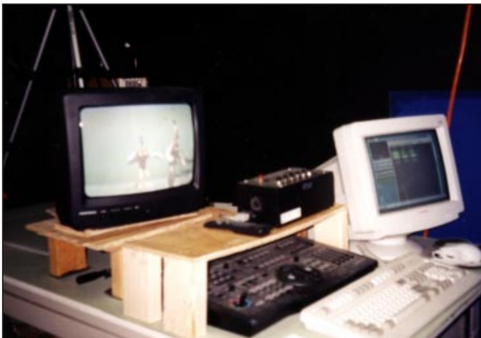
The Neverhood's digital animation set-up includes a digital camera, a capture board, an Animation Toolworks Video Lunchbox, a digital video mixer, a monitor and a multi-giga-byte computer to store images.
