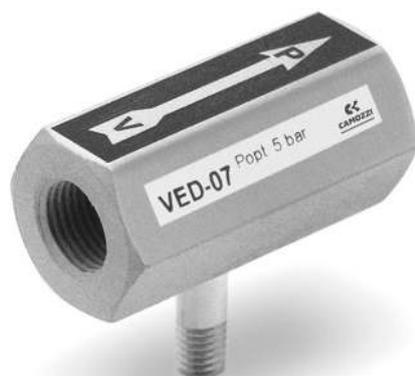
These ejectors are used for direct installation inline between the suction pad compressed air supply. This substantially reduces the volume to be evacuated and allows therefore shorter cycle times.
