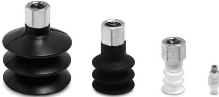
Series VTCN bellows suction pads (2,5 folds) have a rugged design and consist of a nipple and rubber part. The nipples are inserted directly into the rubber part. The rubber parts can also be ordered separately without nipples as spare parts. Materials: NBR or Silicone
