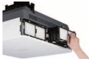
Air filter replacement
