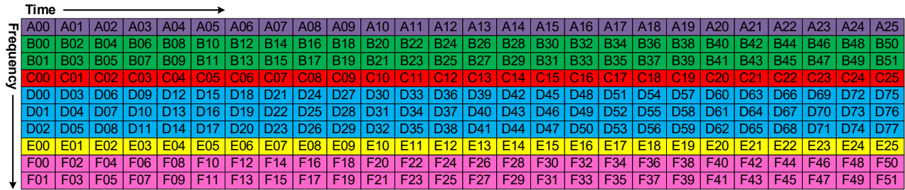
Figure 7.24 Example of frequency division multiplexing of PLPs.
