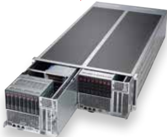
FatTwin™ 2 DP Nodes, 6 GPU/Coprocessor per Node, Front I/O, 16 DIMMs
