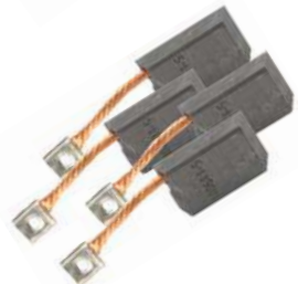
Part Number - 093585 Brush Set (Set of 4) 0.405 D x 0.855 W x 1.430 L
