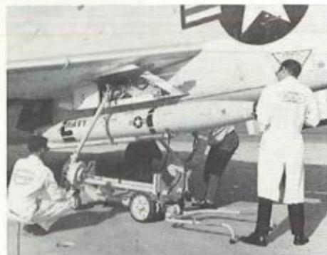
**This Beech AQM-37A target missile** is used as the test-bed for the first U.S. hybrid rocket propulsion system, developed by United Technology Center, Division of United Aircraft Corporation. During first tests the missile was sent to altitudes up to 80,000 feet, to speeds in excess of 2,000 mph and demonstrated its maneuverability at supersonic speeds—exactly as planned.
