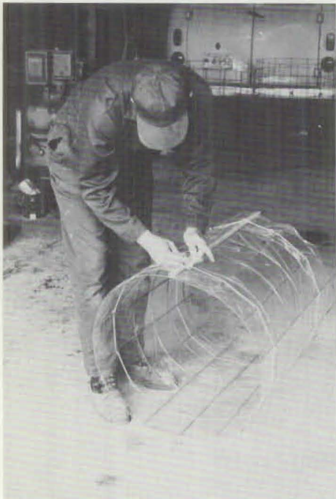
Figure 1: A sheet of plastic is wrapped around a welded wire mesh cage. The sheet can be held taut by wrapping its end around a stick secured with strings.
