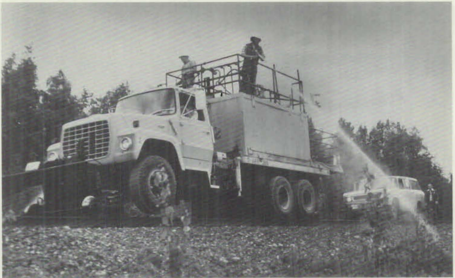
Figure 1: Spraying the right-of-way of the Alaska R.R. near Wasilla. The truck is adapted to ride on rail or highway and a boom may be fitted to spray both sides of the track.
