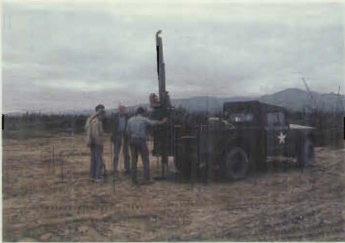
Figure 1: The Giddings soil probe mounted on a 1 1/4 ton munitions truck being prepared to drill a deep core.
