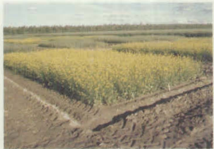
Figure 3: Each subplot was surrounded by a ditch to catch runoff water. The ditches were dug after the plots were seeded using a small one-bottom mold board plow pulled by a garden tractor.
